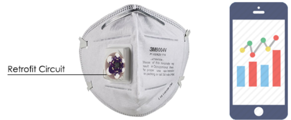
Figure 2: A representative figure showing the retrofitted mask and the associated mobile application.
